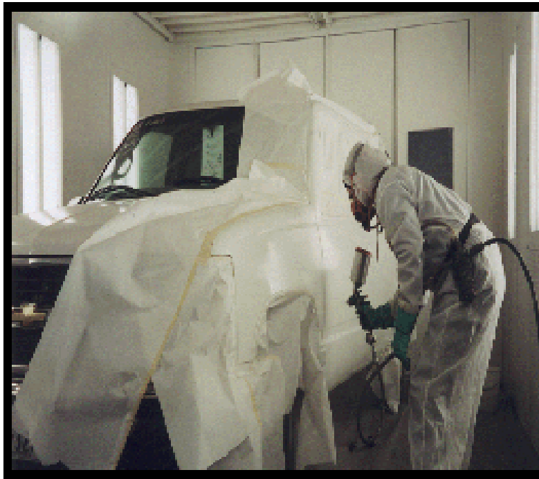
Figure 1. Personal protection equipment used while spraying in the paint booth.
